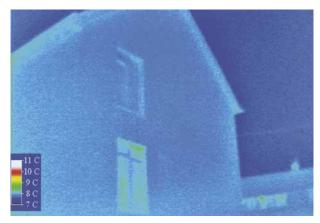
The image above shows a Kingspan TEK® Building System gable wall with a relatively even surface temperature. Very little thermal bridging can be identified. There is also no visible air leakage at the verge. It should be noted that the rooms behind the wall are well heated which further displays the well insulated nature of the construction.
